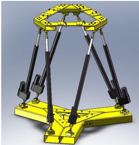
Figure 1: solid model of typical Stewart platform manipulator [10]
